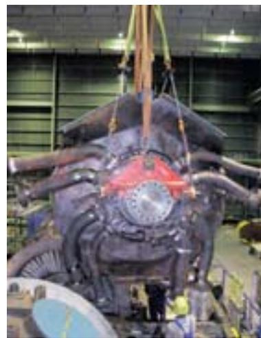
**3** Assembly of the radial turbine before installation.
