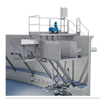
The scraper can be equipped with a peripheral surface scraper, supported from the bottom scraper arm. The surface scraper collects the surface foam in the scum box unit which is attached to the concrete wall. The sludge is removed from the scum box through pipes in the concrete wall.
