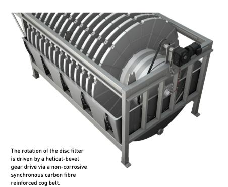
When the water level inside the filter discs increases to a pre-set point, the filter rotor starts rotating and the backwash of the filter cloth starts. The high-pressure backwash spray nozzles remove the accumulated suspended solids into the reject trough inside the filter. The suspended solids are discharged by gravity.
