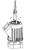
Figure 14: Cooling jacket removal (J 205)
