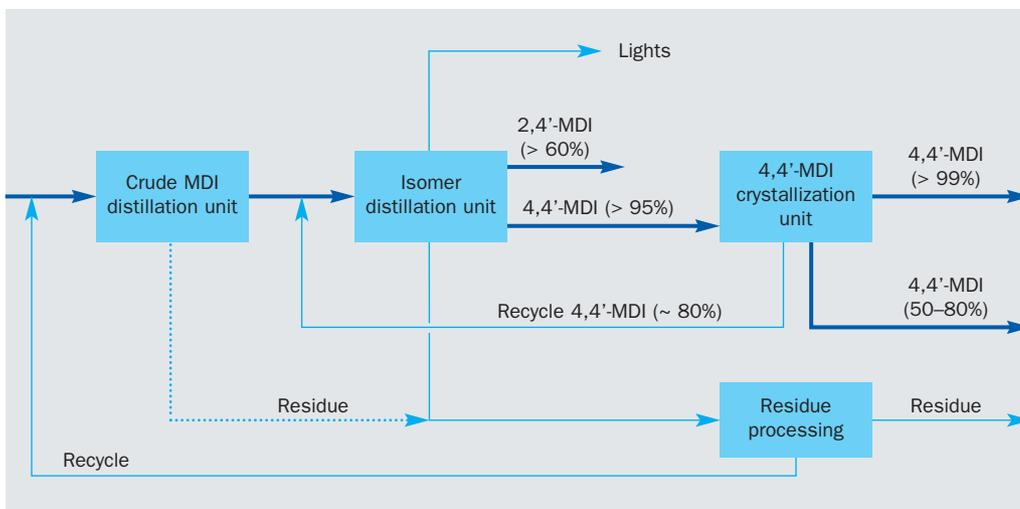
**3** Flow of material by the new hybrid process for the purification and separation of MDI-isomers. If one of the process units is already available in an existing plant, the capacity can be expanded by means of a retrofit.
