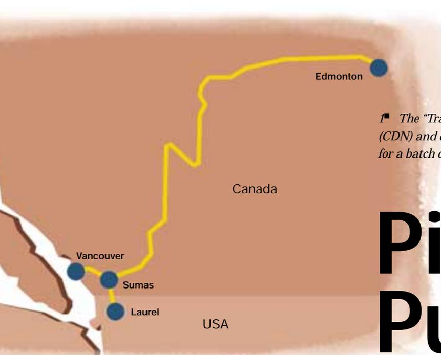
1<sup>■</sup> The "Transmountain Pipeline" starts at Edmonton (CDN) and ends at the Pacific coast. It takes 196 hours for a batch of oil to transit the pipeline.
