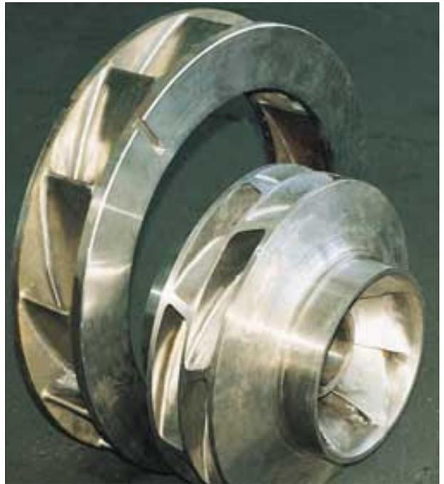
5<sup>■</sup> A diffuser (left) and an impeller (right) of a HSD pump: The vanes at the impeller discharge have a twist of 20 to 30 degrees. This is one of the factors that facilitate smooth pump operation.
