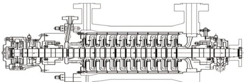
The new Sulzer cartridge in the existing barrel casing
