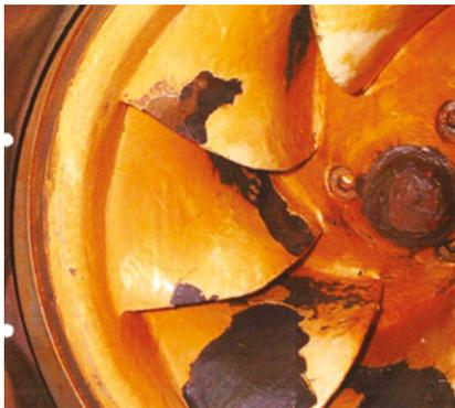
The original cavitation damaged impeller
