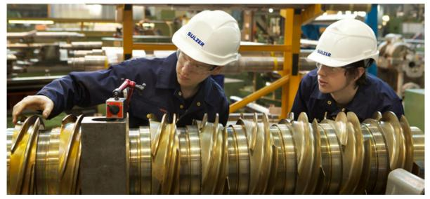
Dunbar multiphase pump rotor on the balancing machine
