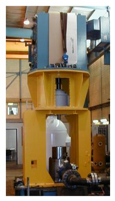
Dunbar multiphase pump package during Factory Acceptance Test (FAT)
