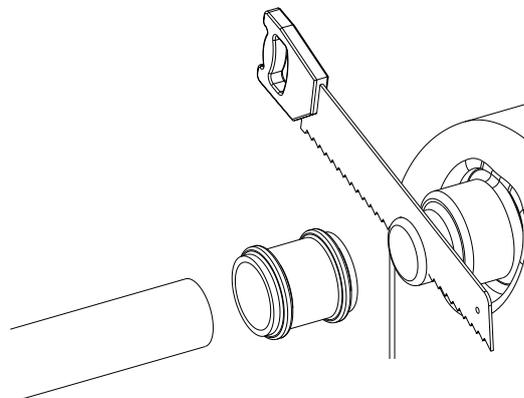
Figure 12: Opening the connections on the collection tank
