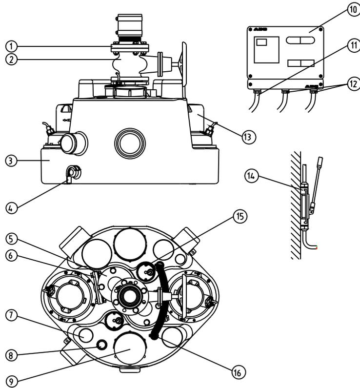
Figure 4: Design of the lifting station Sanimat 1002 and Piranhamat 1002
