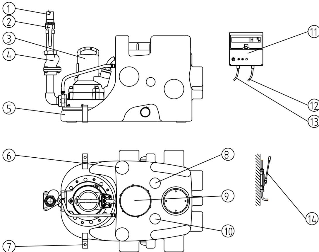
Figure 5: Design of the lifting station Piranhamat 701
