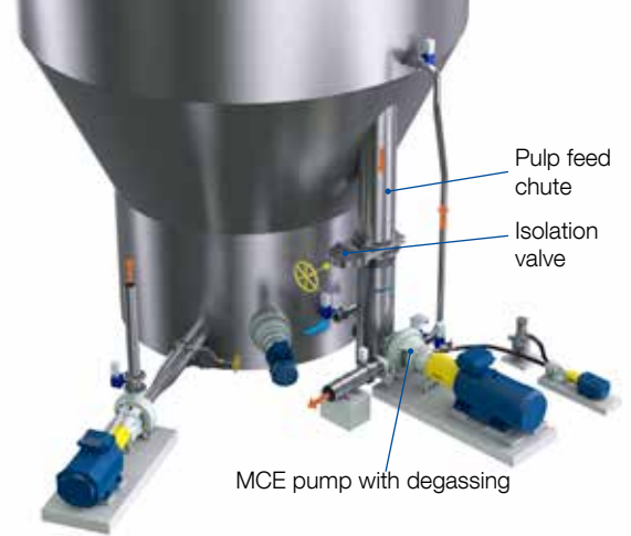
Fig. 23. MC parallel pumping system arrangement.
