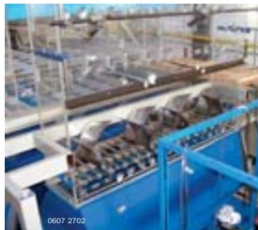
**6** Experimental setup for the evaluation of the Contour mixers. The variations in speed and droplet density resulting from the flow calculations and the experiment were in good agreement.
