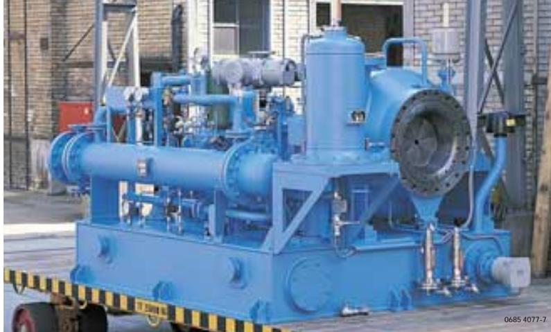
3 This single-stage radial turbocompressor from Sulzer is suitable for the compression of 1-butene or isobutane, for example.
