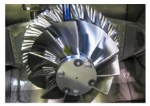
The new impeller vanes were manufactured from a solid piece of chrome molybdenum vanadium steel using 5-axis vertical milling machine
