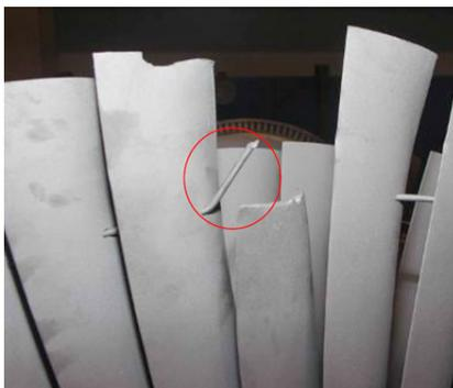
Blade failure caused by vibratory fatigue
