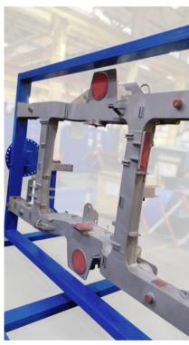
Bespoke 'gyroscope' frames fabricated in-house to allow bogie workpieces to be rotated and held in place for ease of access to areas in need of repairs
