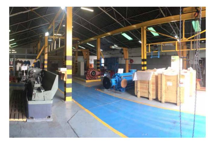
The workshop in Chingola does refurbishment of up to 10 stage pumps and underground air drills (a new Sulzer product line). It allows for sandblasting, spray painting, welding, machining, assembly and balancing of Sulzer pumps and pump components.
