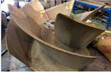
Circulating water pump impeller for power station
