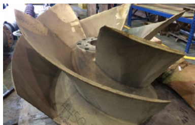
Circulating Water Pump Impeller for Power Station
