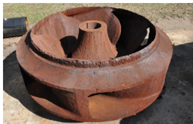
66" Impeller for Dewatering Service
