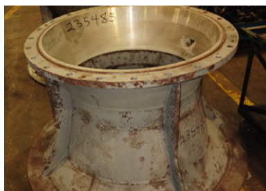
Fabricated Stainless Steel Suction Bell
