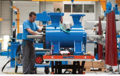
Left to right: Vertical CNC lathe Assembly of a boiler feed pump Training centre
