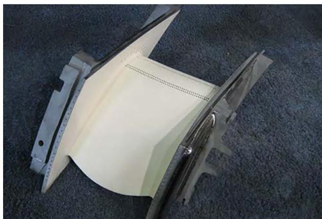
Gas turbine vane repair
