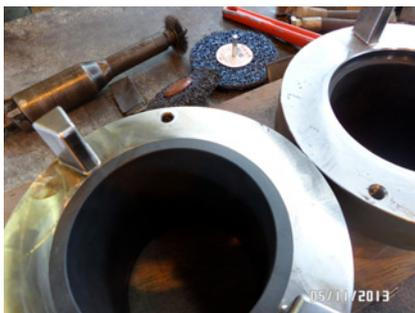
Comparison of throttle bush before and after failure with heat effected zones
