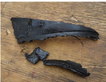
Remains of polymer wear parts after failure
