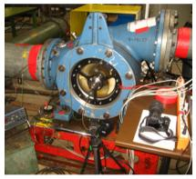
Test on a scale down model of a boiler feed water pump with diffuser 测试一个带有新导叶的、缩小尺寸比例的锅炉给水泵
