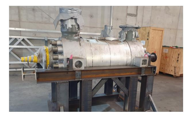
The pump was removed and transported to Sulzer's service center in Jänschwalde to enable the necessary repairs to be completed
