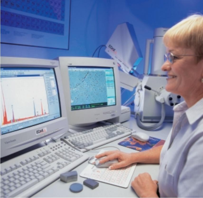
2<sup>■</sup> *New equipment purchased for the contract in the Middle East ensures a qualitatively high standing repair. For instance, a scanning electron microscope with EDAX (Energy Dispersive X-Ray Spectroscopy) capability analyzes the properties of every component and helps also in evaluating the best repair method for them.*
