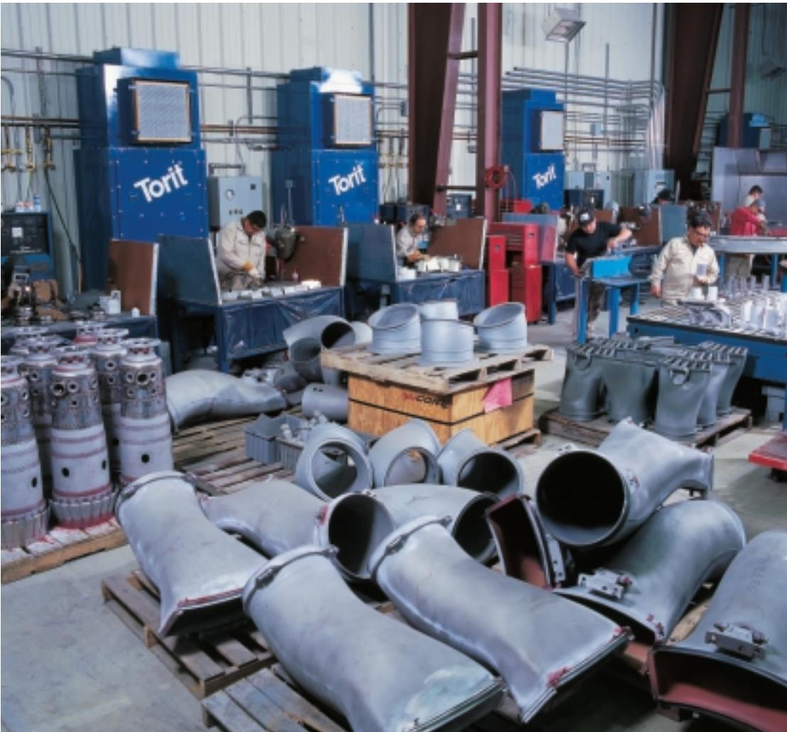
4<sup>■</sup> Special environmentally protective filters at welding stations allow to remove dust, debris, and foreign material in the environment, which reduces contaminations in the repair and also improves the quality of life for the co-worker.
