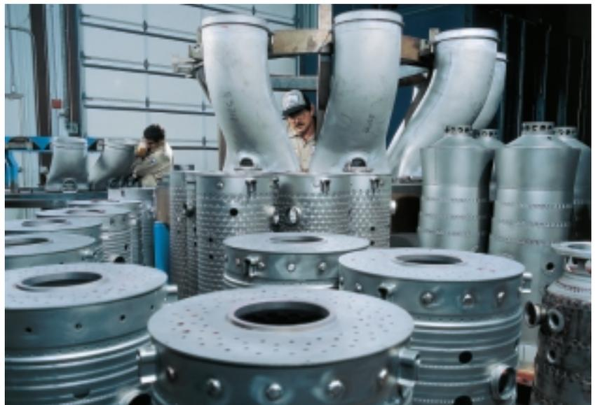
3<sup>■</sup> *A device called “Texas initiative” shown in the background was invented by Hickham to simulate fitting of transition pieces into the nozzle because transition pieces are often sent without the nozzles to verify against.*
