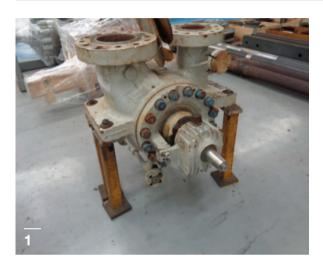
Having achieved excellent reliability for almost 20 years with very little change in pump performance, engineers on an offshore platform detected accelerated abrasion rates on one of its MOL pumps during monthly ultrasonic testing (UT). An expanded oil field had led to a change of application, causing a marked increase in sand and particles passing through the pump. The IOC required a rapid pump repair and upgrade while a standby operated as the main asset to secure oil transfer uptime.
