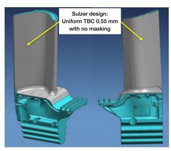
In addition, the weak design feature of the letter box has been removed and the squealer tip has been redesigned to obtain an optimal stress distribution in the tip section, without affecting the cooling integrity of the component.
