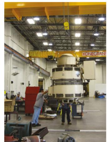
Windings of quad-coat Essex magnet wire makes us virtually unique in the USA. The wire has twice the number of coats of resin as the industry-standard “heavy armored” wire, so the resin thickness is twice as great.
