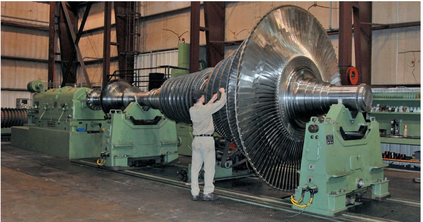
**1** A large steam turbine for a power generation facility undergoing a low-speed balance at the workshop. This low-speed balance stand has a capacity for rotating elements to 50 tons at 500 rpm.
