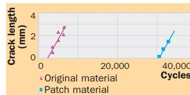
**3** Results of LCF analysis of nickel-base superalloys: the growth of cracks during experiments.
