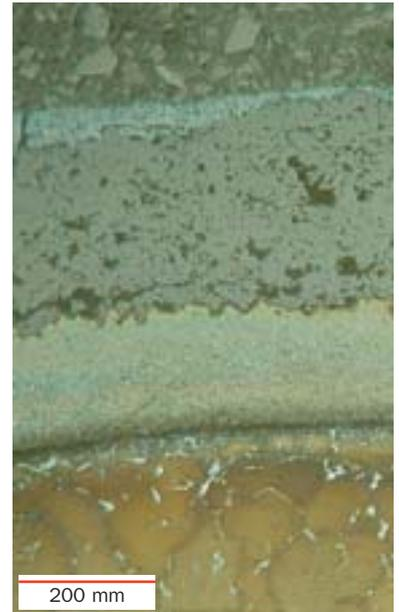
6 The coating microstructure shows no indications of damage after a full operational cycle.
