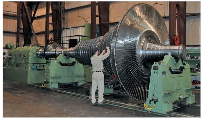
A large steam turbine for a power generation facility undergoing a lowspeed balance at the workshop. This lowspeed balance stand has a capacity for rotating elements to 50 tons at 500 rpm.
