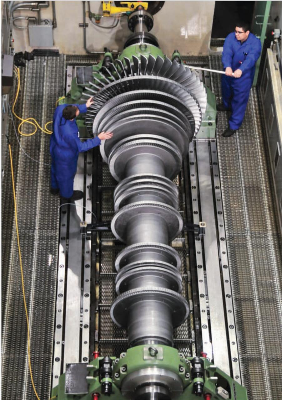
(3) High-speed steam turbine, typical of the type requiring high-speed balancing.
