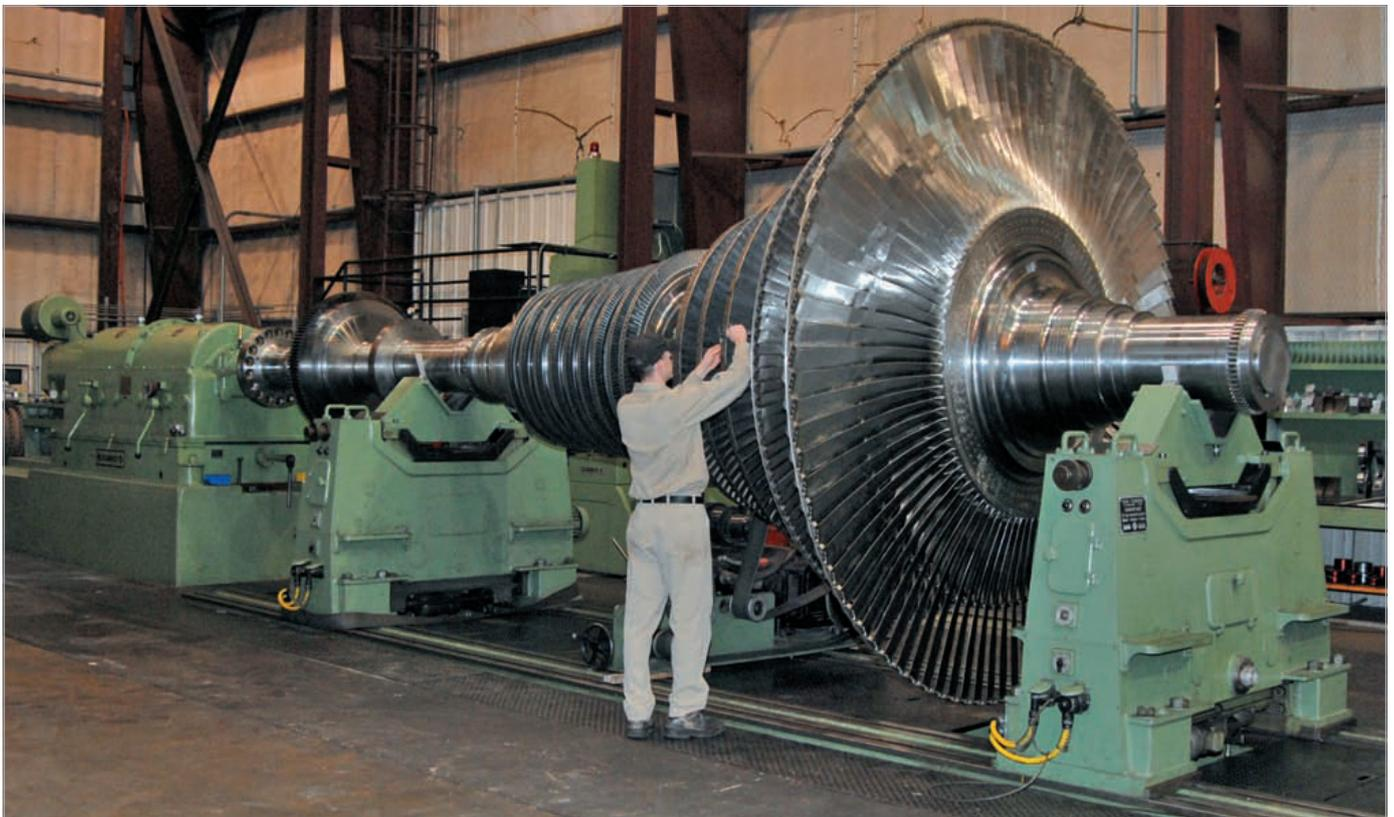
*A large steam turbine for a power generation facility undergoing a lowspeed balance at the workshop. This lowspeed balance stand has a capacity for rotating elements to 50 tons at 500 rpm.*
