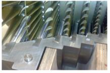
Checking of blade clearances before finalizing..
