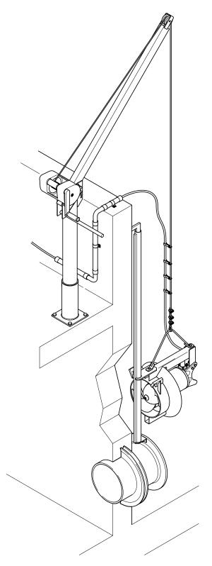
Figure 19. Installation example with Sulzer lifting unit 5 kN
