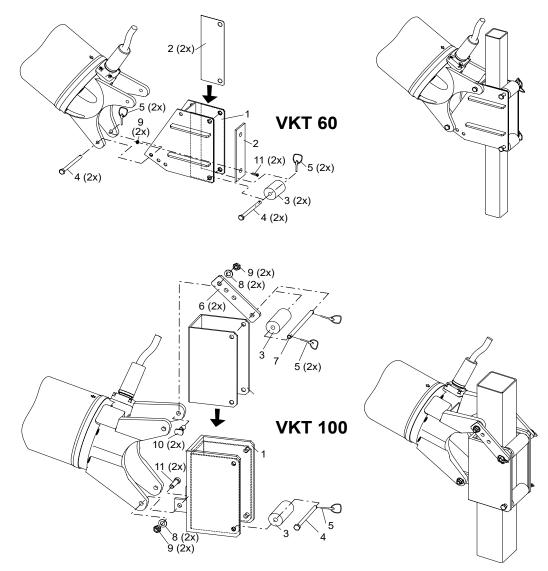
Figure 17. Closed bracket with vertical swivelling
