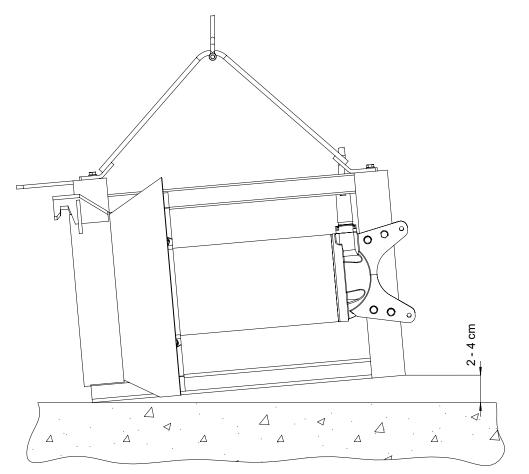
Figure 22. checking installation angle of pump
