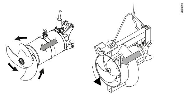
Figure 29. Checking direction of rotation
