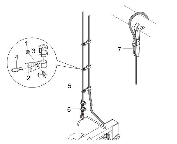
Figure 21. Securing and positioning of the motor connection cables of the RCP
