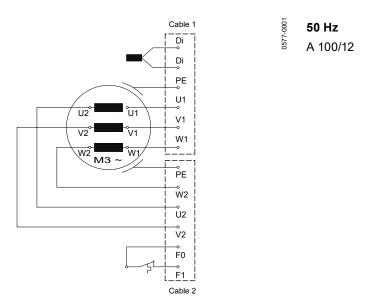
Figure 26. Two power cables with integrated control leads
