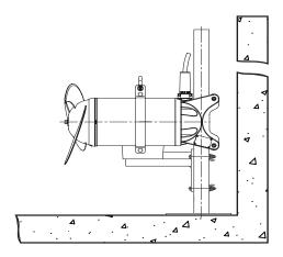
Figure 14. Fixed installation with vibration damper
