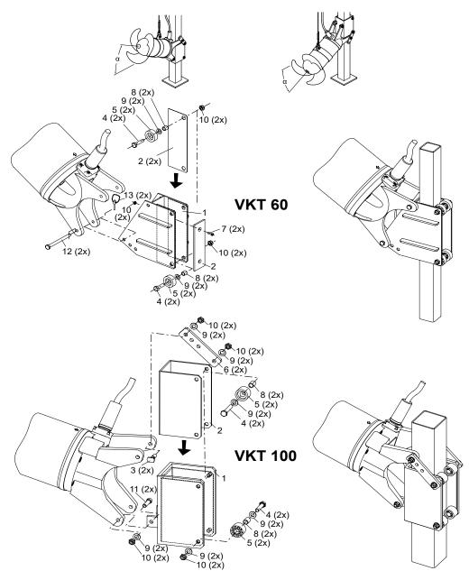
Figure 16. Open bracket with vertical swivelling
