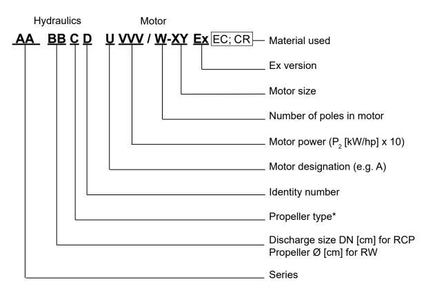
\*Propeller type: 1 = Mixing propeller (only without flow ring); 2 = 2-blade thrust propeller; 3 = 3-blade thrust propeller;
