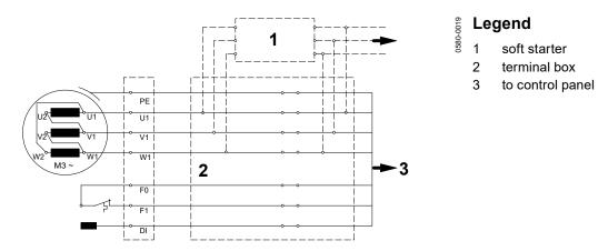
Figure 27. Wiring diagram with soft starter (option)
