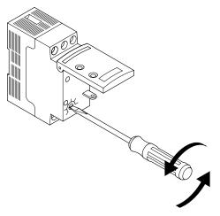
Figure 28. Testing and adjustment of soft starter
