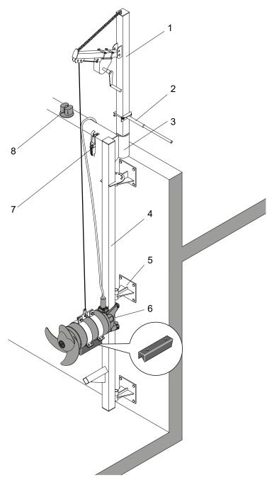
Figure 12. Installation example with alternative fixing possibilities
