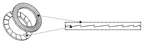
Figure 10. Correct fitting position of the Nord-Lock® securing washers
