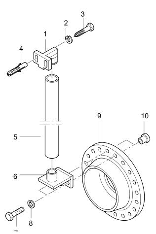
Figure 20. Guide tube installation
