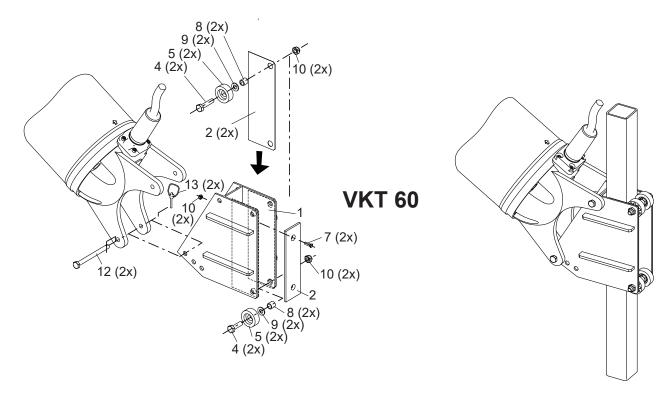
Figure 15: Open bracket with vertical swivelling
