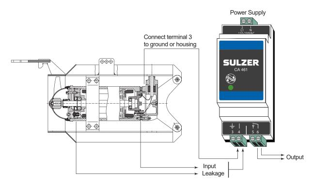
Figure 21: Sulzer leakage control type CA 461
