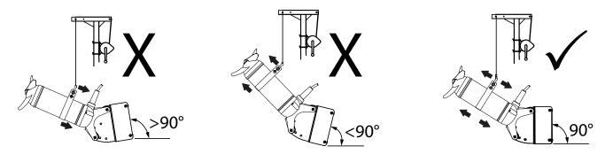
Figure 17: Setting up with fully mounted bracket
