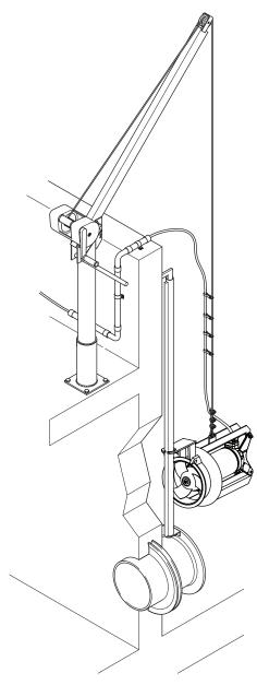
Figure 8: Installation example with Sulzer lifting unit 5 kN
