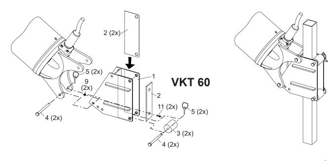
Figure 16: Closed bracket with vertical swivelling
