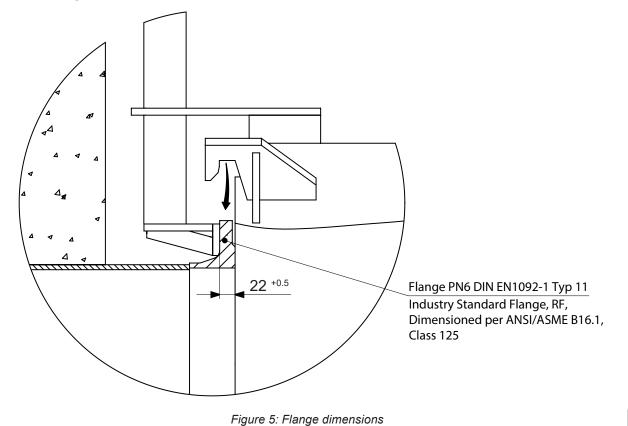
ATTENTION Before installing the recirculation pump, check the dimension of the flange. Make sure that the dimension specified in the drawing is adhered to, otherwise the flange will need to be reworked.
