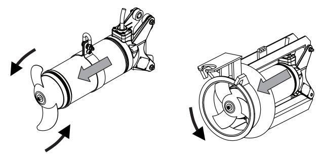
Figure 23: Checking direction of rotation
