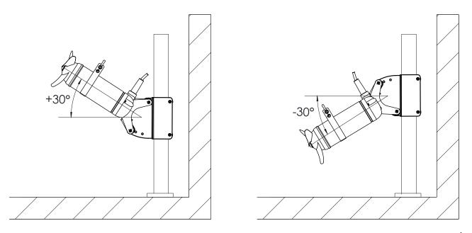
Figure 18: Vertical adjustment on the guide rail
