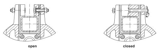
Figure 14: Open bracket/closed bracket
