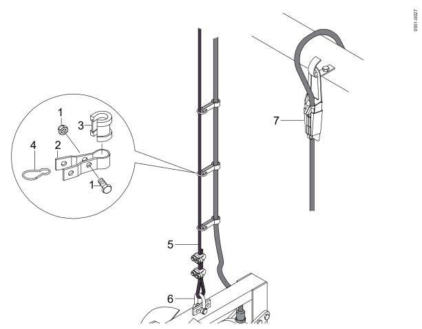
Figure 12: Securing and positioning of the motor connection cables of the RCP
