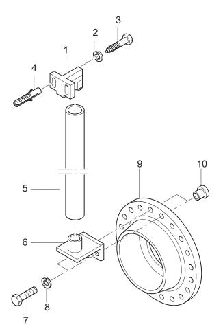
Figure 9: Guide tube installation
