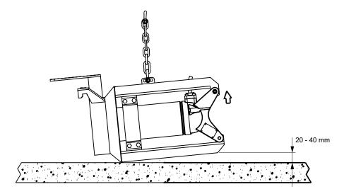
Figure 10: Checking installation angle of pump
