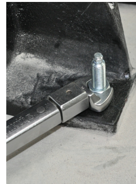
Figure 9d: Tighten nut
