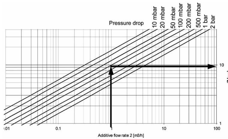
Fig. (12). Suggested guidelines for selecting the hole diameter for the additive flowrate.
