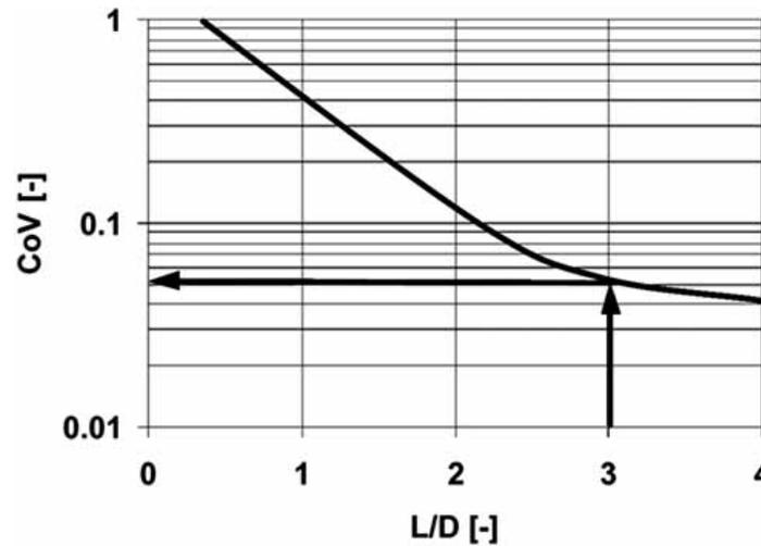
Fig. (13). Suggested guidelines for evaluating the coefficient of variation as a function of the pipe dimensionless length.
