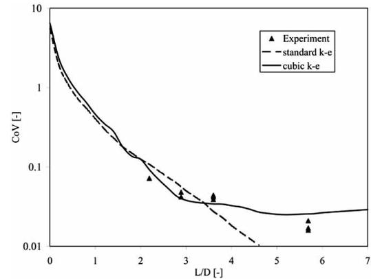
**Fig. (8).** Mixing in pipe after outlet of the CompaX mixer comparison between experimental data and CFD results.
