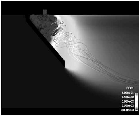
**Fig. (5).** A detail of the CFD simulation performed by Fleischli and Suhner [12] (STAR-CD, Standard k-ε model, incompressible flow, Conditions: Air, P = 1 bar, T = 20°C, main flow = 10m/s, additive = 23m/s, flow ratio 1:300).
