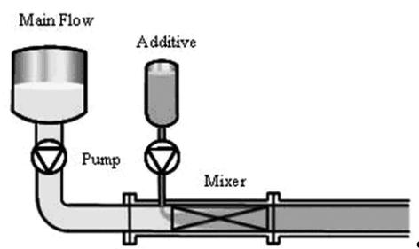
Fig. (1). A schematic diagram of the mixer.
