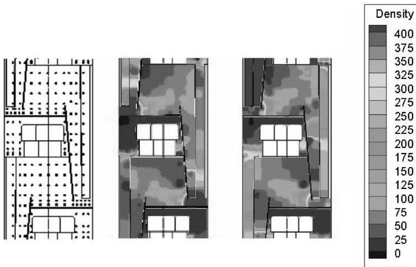
**Figure 3.** Gamma-scans for iC4/nC4 mixture at 11bar, tray spacing = 450 mm under total reflux conditions. Points in picture on the left show 'scan points'. The vapour load increases from left to right from  $C_f = 0.08$  m/s to  $C_f = 0.11$  m/s ( $C_f$  = based on total column cross sectional area).
