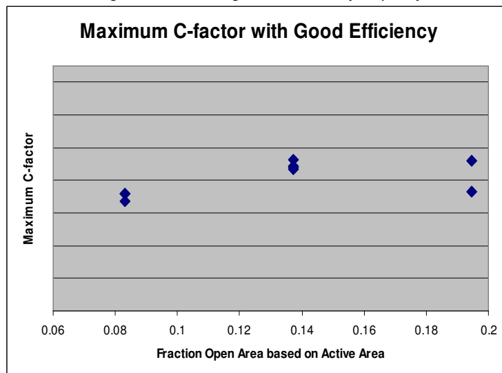
Figure 5 – Open Area effect on Tray Capacity
