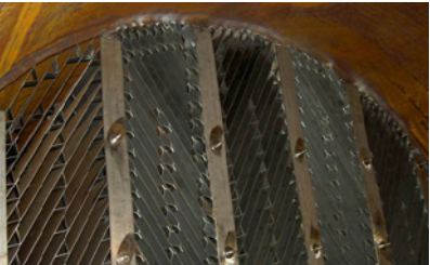
Mellaplate coalescer for the top receiver
