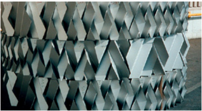
SMV packing for the catalyst stripper
