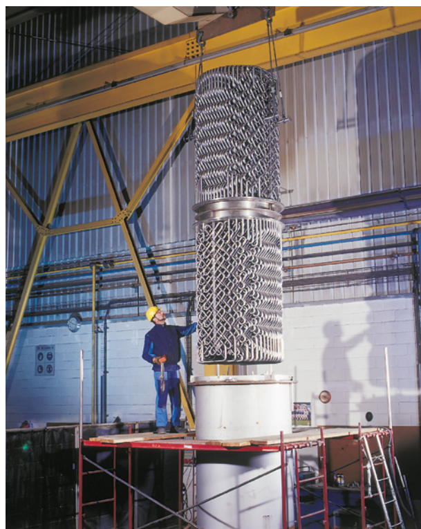
SMR mixer-reactor for heat exchange in exothermic reactions for the chemical/petrochemical industry
