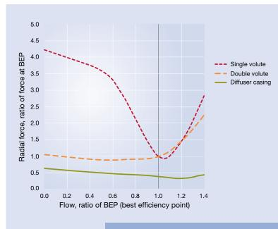
Fig. 4: Radial thrust comparison
