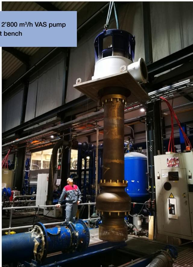
of operating a single pump designed for the total capacity (i.e. tank lay-out, single downstream line, etc.). The initial requirement considered a single pump in operation with a flow rate of 2'600 m<sup>3</sup>/h.
