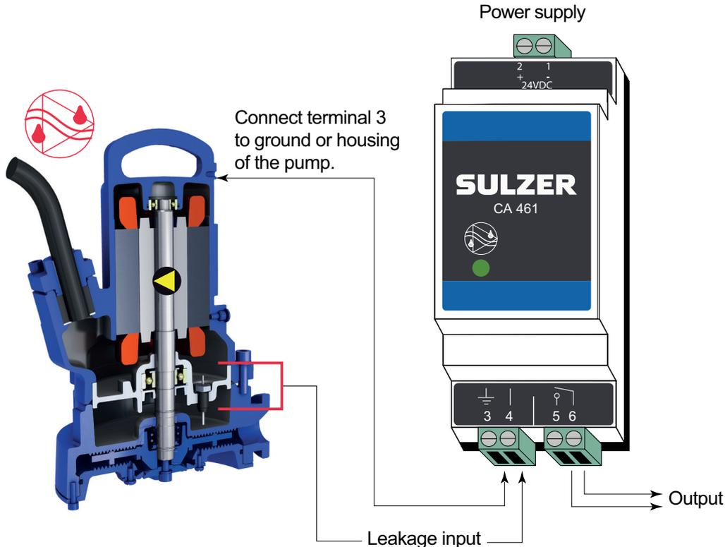
Sulzer leakage control type CA 461
