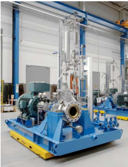
Sulzer ZF pump for HTF overflow service in final inspection
