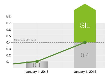
MEI, the minimum efficiency index for standardized water pumps, was set up to be  $\geq 0.4$  since the beginning of 2015. This means that at present 40% of the pumps on the market do not comply.
