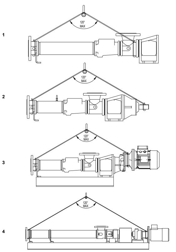
Figure 1. recommended lifting points
