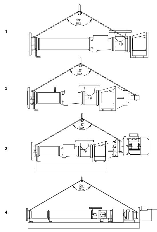
Figure 1. recommended lifting points
