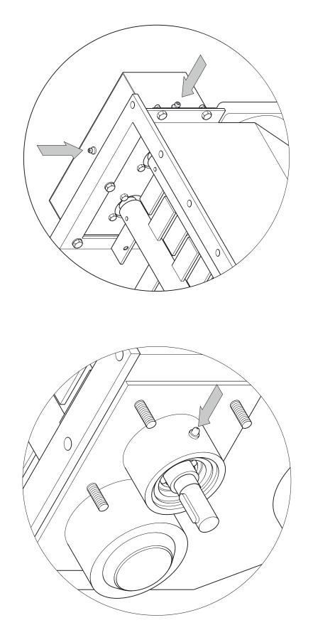
Above positions should be generously charged with the recommended grease using the grease nipples provided.
