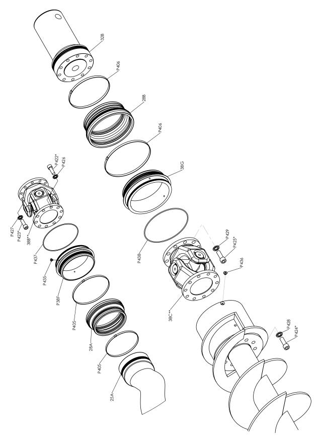
\* P422, P423, P424, P425, P435 and P436 to be fitted using Loctite 242 applied to the threads.
