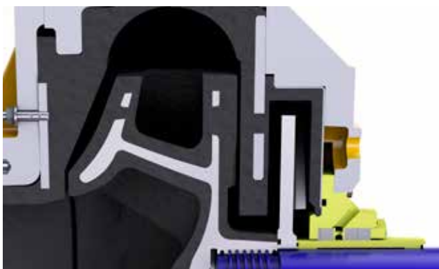
Separate and removable suction plate (from size 200).
