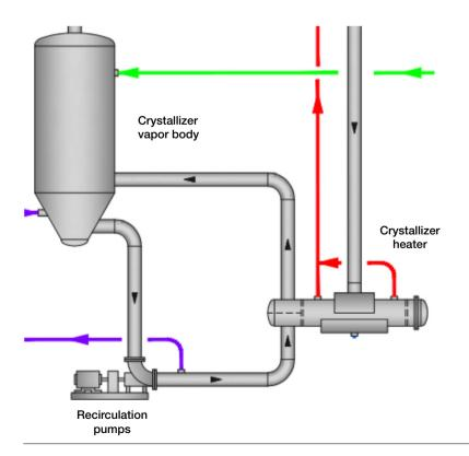
Typical evaporator heat exchanger circulation loop (figure 1)
